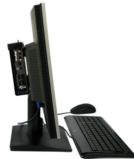
Linutop placed on the back of a flat panel, with the monitor mounting bracket accessory
